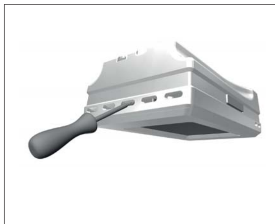
Illustration 2: Removing the front cover
